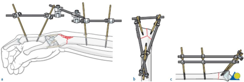
*a Bridging external fixation. Indirect reduction using ligamentotaxis, with a tube-to-tube construct.*
